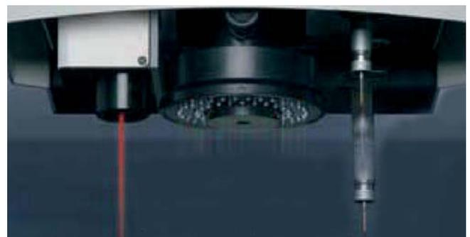
*Measuring head of the PMS Series with a CCD matrix camera, a TP 200 touch probe which retracts after use and a conoscopic measuring laser.*
